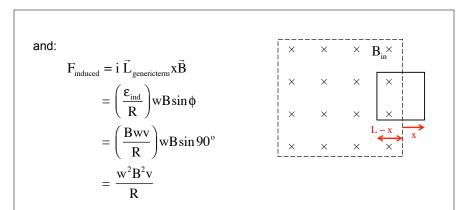
As the coil is trying to exit the magnetic field moving to the right, the induced force due to the induced current's interaction with the external magnetic field will be LEFTWARD.
