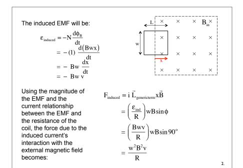
b.) Once the coil is completely inside the magnetic field, there is no longer a CHANGING MAGNETIC FLUX, which means there is no longer an INDUCED EMF or subsequent INDUCED CURRENT, and as such there will be no magnetic force present on the coil.
